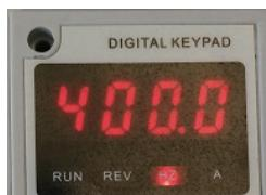
Fig.3 The VFD is standby and showing preset frequency 400Hz
