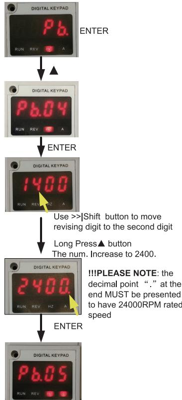
Fig.2 Step to set the Rate. Speed in PB.04
